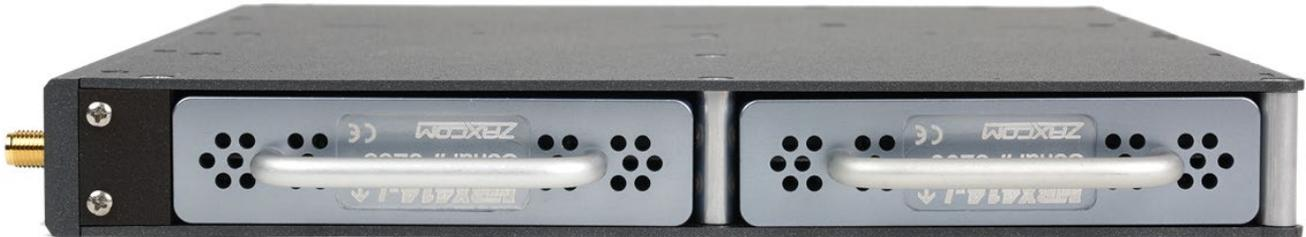
The two MRX receivers slide into the side of the RX-8. The A receiver goes to in the bottom slot away from the front panel and the B receiver goes in the top by the front panel. The arrows on the MRX will need to point to the bottom of the RX-8. Please note if only using 1 receiver it must go in the A slot.
