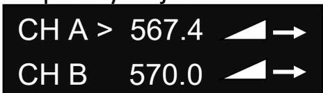
The frequency select menu is where the receive frequencies are set. These frequencies need to match the frequencies that are set on the corresponding transmitters.
