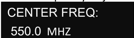
This where the center frequency of the front-end filter is set. The front-end filter is 35MHz wide so frequencies 17.5MHz above and 17.5MHz below the center frequency will be the operating range of the RX-8. MRX receivers will need to operate within the set 35MHz window. If the frequencies aren't within this window the RF performance will suffer. This menu is only available in the A receiver.
