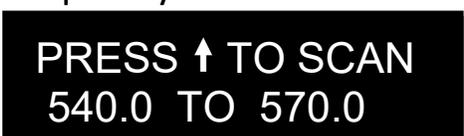
An RF scan is initiated from this menu. After the scan is complete a graphical display of the RF that is present will be shown and the RX-8 will suggest clear frequencies. The frequency can be accepted by pressing the INC key. Pressing the DEC key will skip the first chosen frequency and the RX-8 will suggest another frequency. Please note the RX-8 can scan 30 MHz at a time. Scanning is only available from the A receiver.
