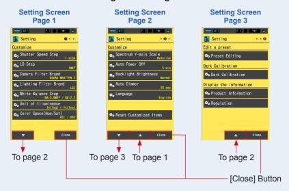
When the [Close] button is touched, the display returns to the Display Mode Selection screen. For more information about how to set and the details of specifications, see "7-1-1 Item List". (▶ P126)
