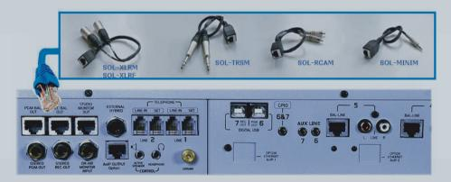
The console uses standard audio connectors, but also incorporates the new technology of RJ45-audio with shielded cable.
