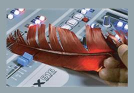
Solidyne is the world only company in offering the new technology of Conductive Ceramic faders of 15 years life. They are easily recognized because of its remarkable softness; it can be moved using a feather.
