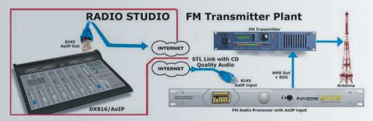
This option allows you to send audio directly from the console to the transmitter plant (STL link) using Internet with the digital audio quality of a Compact Disc.
