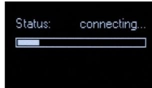
Keep the IR window of the transmitter in front of the IR window of the receiver and, as soon as the connection is done, the receiver will send to the transmitter all the information needed.
