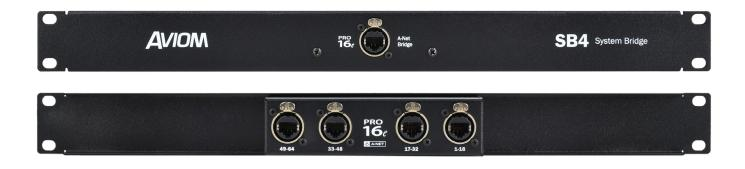
The SB4 System Bridge can be used to combine up to four Pro16® or Pro16e<sup>™</sup> A-Net<sup>®</sup> streams onto a single Cat-5 cable. The rear panel of the SB4 has four A-Net input or output jacks; the front panel features a single A-Net Bridge output. All connections utilize heavy duty locking Neutrik<sup>®</sup> EtherCon<sup>®</sup> Cat-5 jacks.
