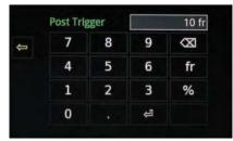
The Post Trigger can be entered in frame count or percentage. The value represents the amount of frames past the trigger point to be stored in RAM
