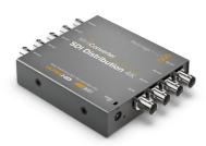
When you need to connect to multiple SDI devices, then Mini Converter SDI Distribution 4K is the perfect solution! Connect a single SDI source to 8 re-clocked SDI outputs with automatic switching between all SD-SDI, HD-SDI, 3G-SDI and 6G-SDI video formats, plus all ASI, ancillary and embedded audio formats.
