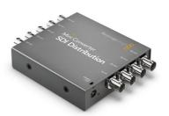
Now you can distribute a single SD or HD-SDI connection to up to 8 different SDI outputs at the same time! You get a true 3G-SDI design with fully re-clocked outputs and automatic switching between all SD and HD formats up to 1080p60. You also get support for all ASI, ancillary and embedded audio formats. Mini Converter SDI Distribution is the perfect SD/HD SDI distribution converter for when you don't need the cost of the Ultra HD model!
