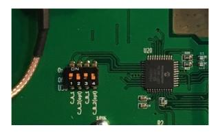
Move up switch C\_A\_A to activate DC feed on coaxial A1 input, move up C B 1 to activate DC feed on coaxial B1 input.
