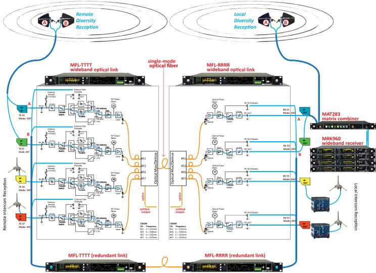
Example of a redundancy link (1-fault tolerance) with automatic failsafe switches
