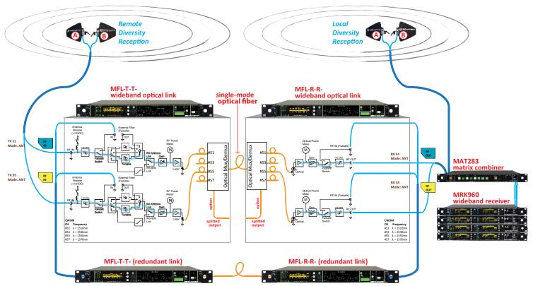
Example of a redundancy link (1-fault tolerance) with automatic failsafe switches
