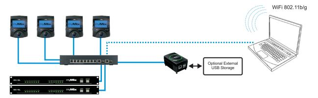
The myMix PLUG interface is connected to the myMix network directly to the network switch. The access to the myMix PLUG web server is either through WiFi or connecting the client interface to the Ethernet network via a CAT5 cable.
