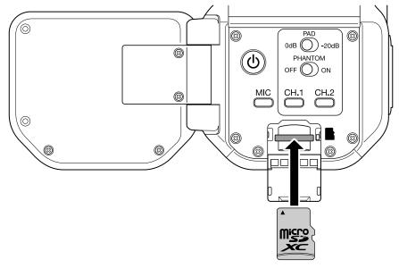
To remove a microSD card, push it further into the slot and then pull it out.
