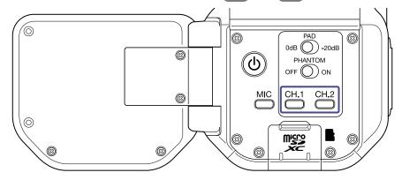
To end the stereo link, press  $\stackrel{\text{CH.1}}{\bigcirc}$  and  $\stackrel{\text{CH.2}}{\bigcirc}$  at the same time again.
