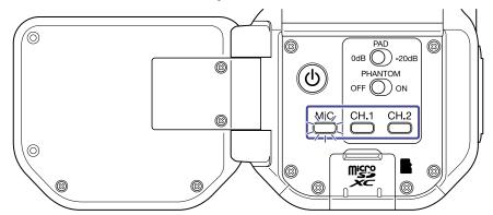
The button indicators for the selected channel buttons light red and you will be able to monitor the signals input on these channels through the Headphone output.
