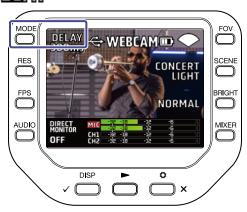
2. Press +10ms or -10ms to adjust the delay time.
