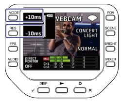
Pressing **+10ms** lengthens the delay time by +10 ms and pressing **-10ms** shortens the delay time by -10 ms.
