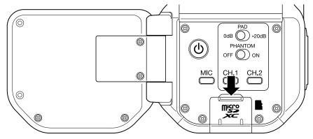
2. Insert a microSD card into the card slot.
