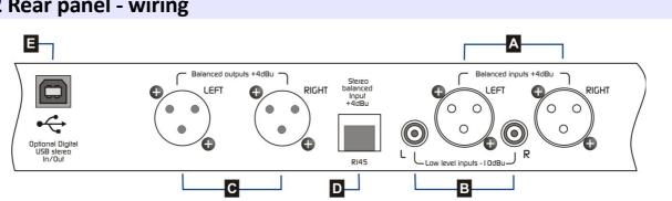
Inputs and outputs are electronically balanced. Use shielded twisted pair audio cables for audio connections (microphone cable). Input and output connectors are XLR. Connect as the following:
