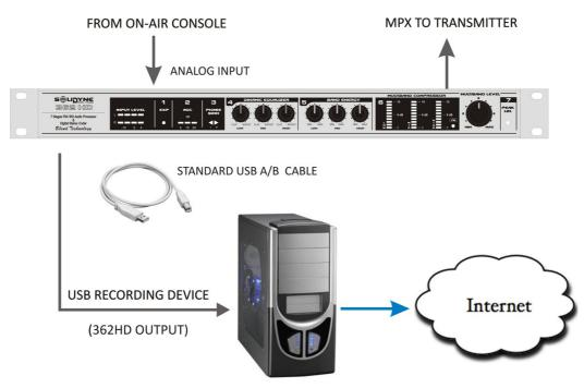
Standard connection for FM with USB for streaming
