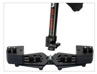
**NOTE:** The adjustment knob should only be tightened by hand. Do not over-tighten it as it could cause thread stripping.
