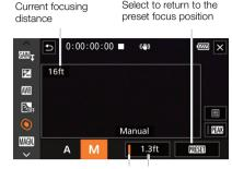
Focus preset button Preset focus (in orange: focus position preset activated)
