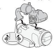
3 Turn the front screw and two rear screws to secure the handle unit.
