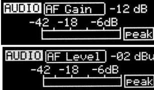
The sensitivity of the audio input is settable between "AF Gain" (measured in dB) or "AF Level" (measured in dBu).
