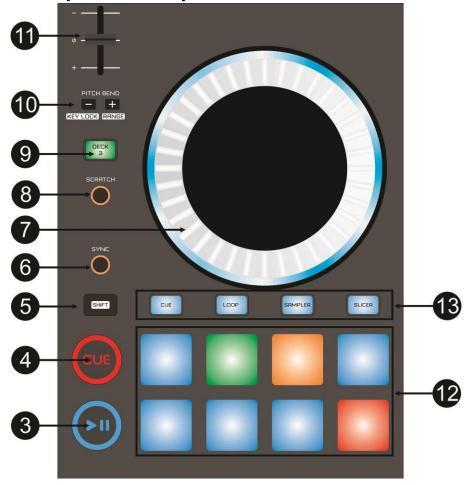
**3. PLAY PAUSE button:** used to start/stop playback of the loaded track. When you use the play button while [SHIFT] is pressed, the song will be automatically synchronized with the other track that is playing.
