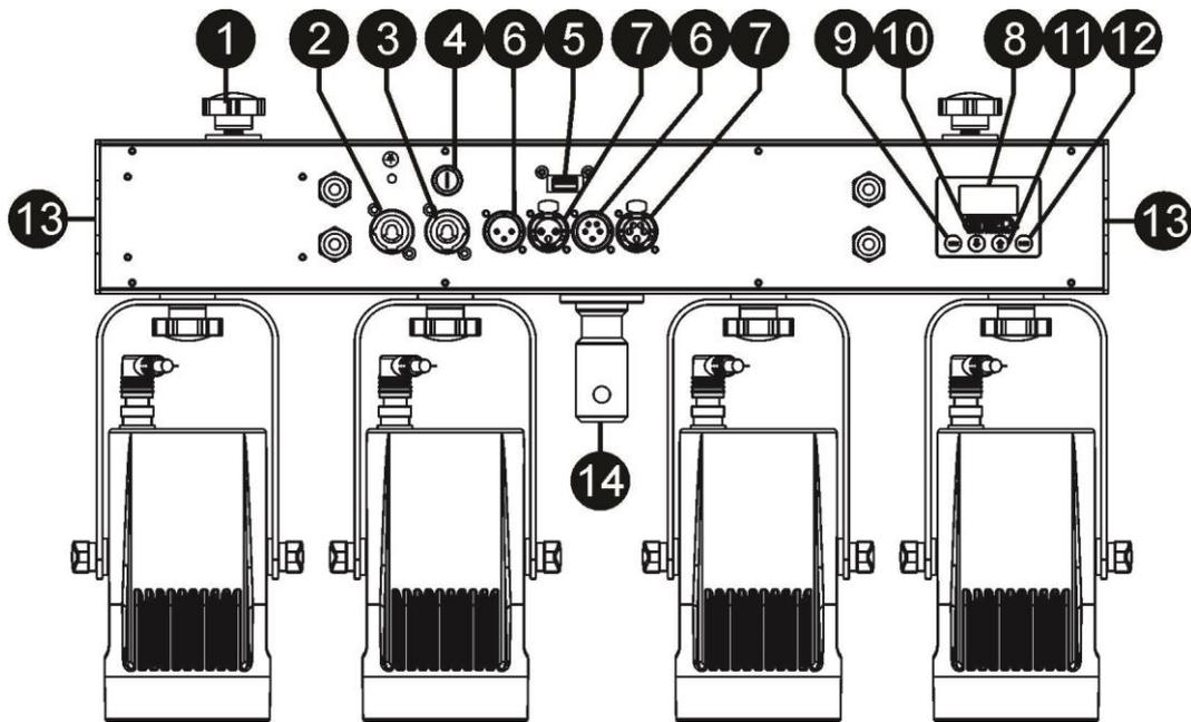
1. **SCREWS:** can be used to fix hanging clamps or other projectors
