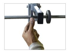
Camera head mount is provided with a knob to control 90° tilt movement of camera. Loosen knob for free tilt movement of camera and tighten it to lock movement.
