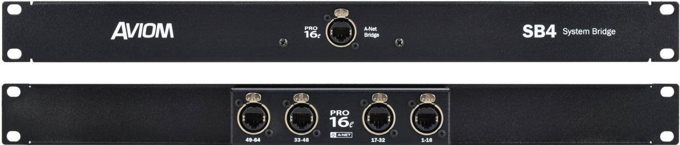
The SB4 System Bridge can be used to combine up to four Pro16® or Pro16e™ A-Net® streams onto a single Cat-5 cable. The rear panel of the SB4 has four A-Net input or output jacks; the front panel features a single A-Net Bridge output. All connections utilize heavy duty locking Neutrik® EtherCon® Cat-5 jacks.
