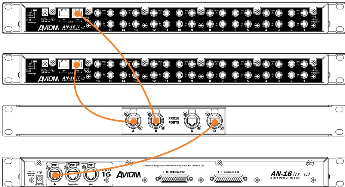
This shows the Cat-5 patching for the 32 x 16 configuration on stage.
