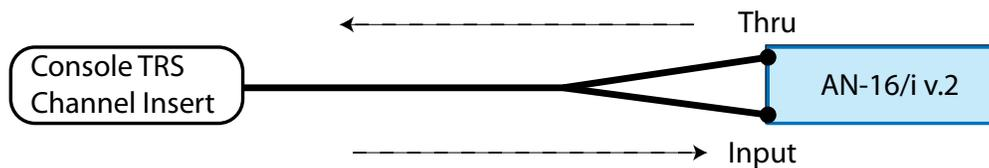
Audio flows from the TRS console insert point into the AN-16/i v.2 and then back to the console.
