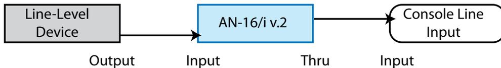
A line-level device is connected to the input module before being connected to the console's line input.
