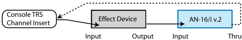
Audio flows from the console insert point into the effect device, then into the AN-16/i, and returns to the console.
