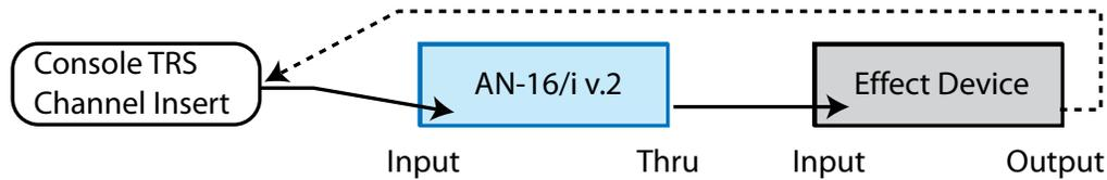
Audio flows from the console insert point into the AN-16/i, then into the effect device, and returns to the console.
