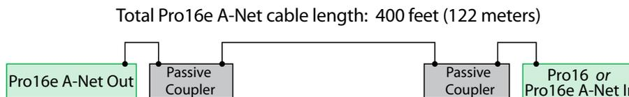
The maximum cable length specification applies to the total cable length between an **A-NET OUT** port on one device and the **A-NET IN** port on the next A-Net capable device in your system.
