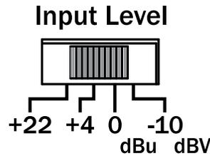
The AN-16/i v.2 has four input level options per channel pair.
