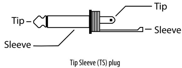
A typical insert cable is wired as seen below:
