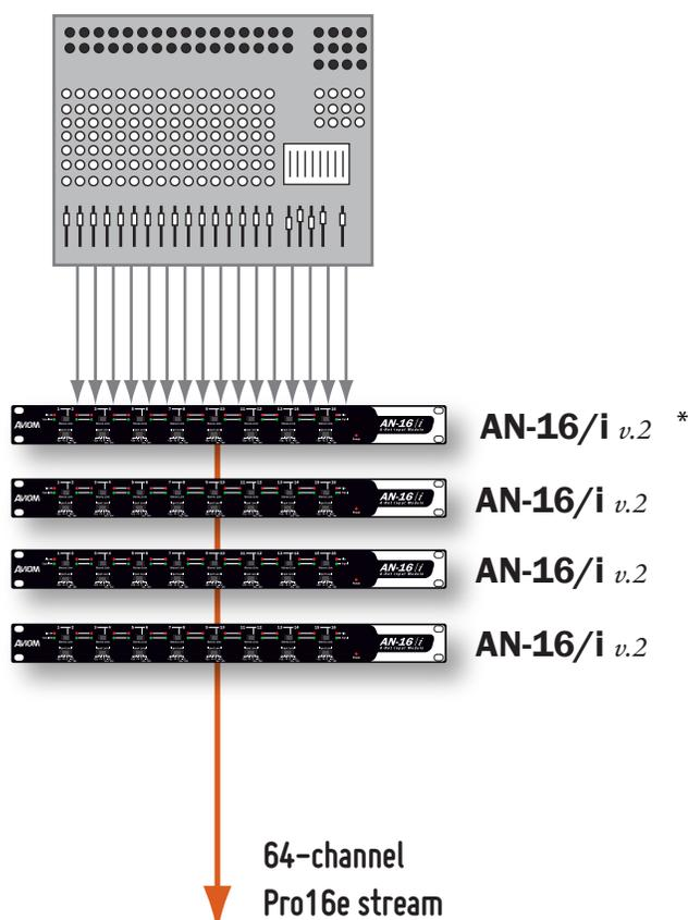
Four AN-16/i v.2 Input Modules can provide up to 64 audio sources for A360 Personal Mixers to select from.
