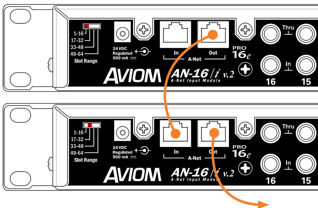
Set the Slot Ranges to 1-16 and 17-32 on the input modules.
