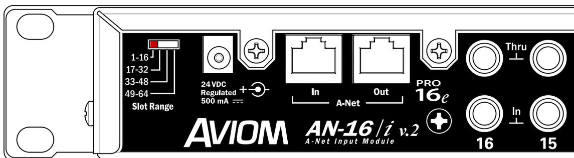
A 16-channel application requires the Slot Range switch to be set to the 1-16 position.
