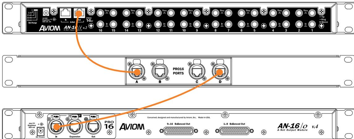
Cat-5 connections on stage for the 16 x16 digital snake are shown.
