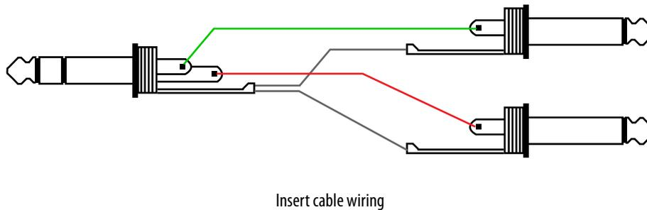
Using a TRS insert, the DSP effects device would have the insert Send cable plugged into its input and the insert Return cable plugged into its output. This wiring completes the signal loop without interrupting the audio being played through the console.
