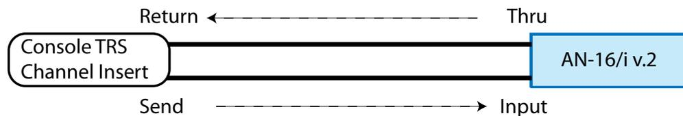
Audio flows from the Send jack of the console insert point into the AN-16/i v.2 and then back into the console via the Insert Return jack.
