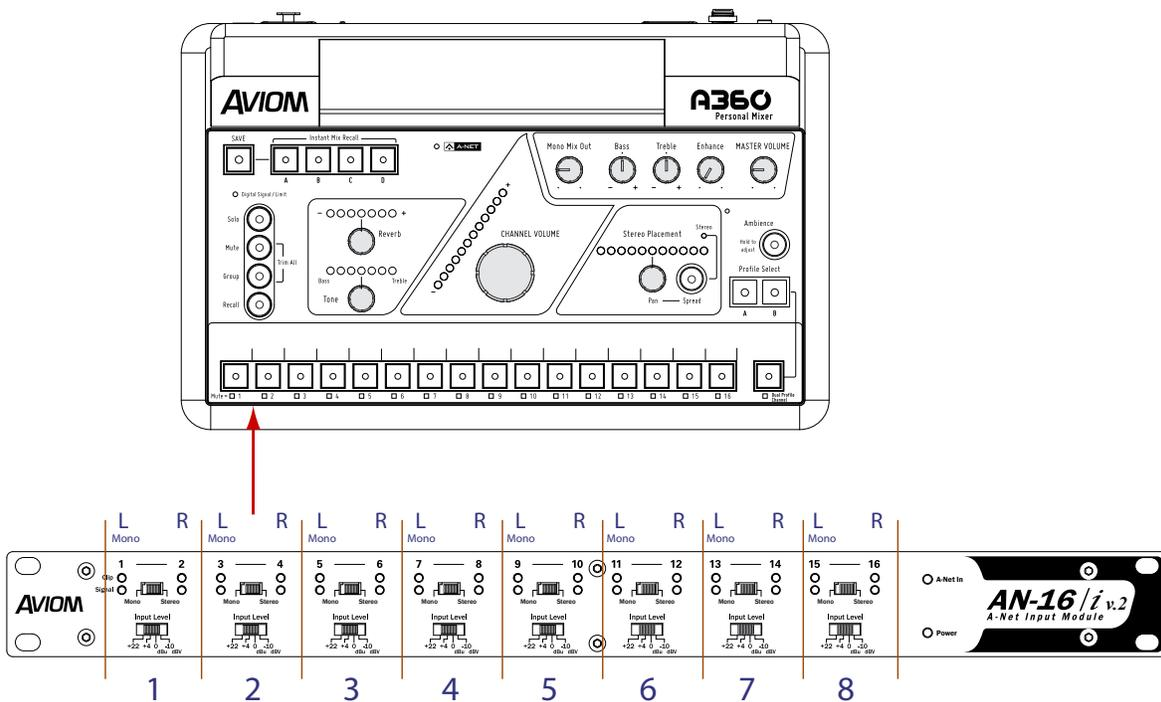
Inputs are treated as stereo pairs; audio sources connected to input jacks 3 and 4 become the second stereo pair when linked. They map to channel button 2 on an A360 or A320 Personal Mixer.
