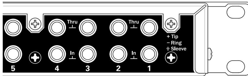
Input and Thru jacks are TRS balanced.
