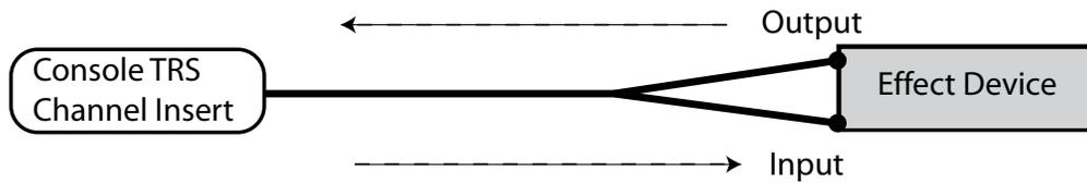
Audio flows from the console insert point into the effect device and then back to the console using a Y-cable.
