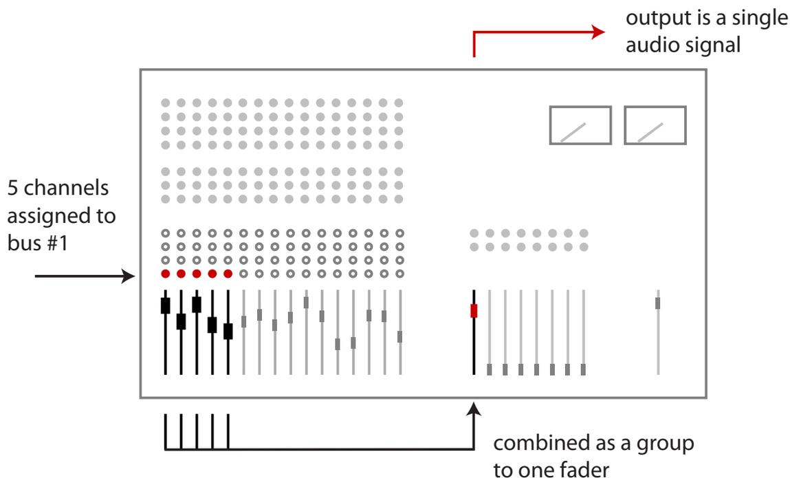
Five channels are combined and can be output as a single channel of audio.
