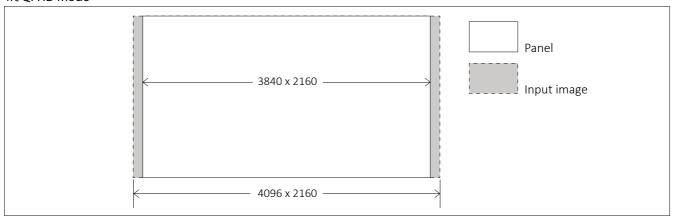
The LCD panel resolution of OBM-U240/U550L is QFHD(16:9) 3840x2160, so if the input signal is 3840x2160, 1:1 mapping is supported. If the input signal is DCl 4K(1.89:1) 4096x2160, 1:1 mapping is not supported.
