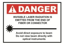
INVISIBLE LASER RADIATION EMITTED FROM END OF FIBER OR CONNECTOR
