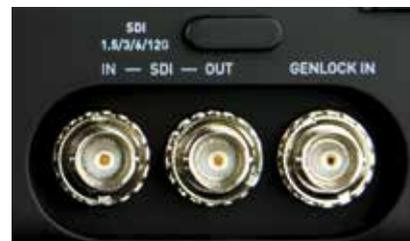
deck is locked to this external reference signal so that the playback output can be synchronized across several playback decks or devices.
