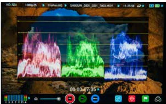
The Waveform Monitor will remain on screen when hiding the overlays ensuring the focus remains on calibrating your image.
