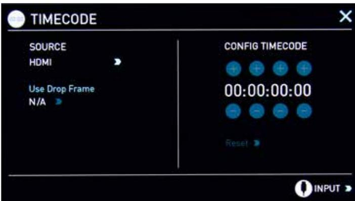
With this setting, the SDI or HDMI input will set the timecode (as long as the source device supports this). The controls to adjust the timecode value are disabled in this setting because the embedded timecode in the SDI/HDMI signal sets the timecode value of the recording. If you want to adjust this please, refer to the manual of your SDI/HDMI input device.
