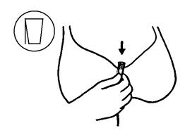
BRA-HOLDER. BRA-HOLDER, SLIDE THE HOLDER OVER THE MICROPHONE AND PLACE THEM ON THE CENTER CORE OF THE BRA. DOESN'T DAMAGE FABRIC AND CAN BE SELF APPLIED BY THE TALENT.
