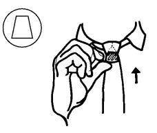
TIE-HOLDER. FEED THE MICROPHONE FROM THE BACK OF THE TIE DOWN THROUGH THE KNOT, APPLY THE TIE-HOLDER TO THE MIC AND PUSH BACK UP INTO THE KNOT.
