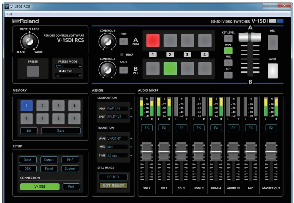
V-1SDI RCS is software designed to control the V-1SDI remotely using a computer. By connecting the V-1SDI and a computer via USB, along with operating the unit from the computer, you can also save and call up settings and perform updates for the system software. Also provided is a backup feature for saving all settings in the V-1SDI to the computer.
