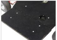
• Take out the allen bolts from dolly base to attach Euro Adapter.
