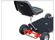
**NOTE:** Chair is adjustable and moves in forward/backward position, to provide more comfort to the operator.
