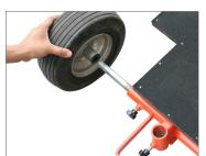
On the provided bushes of wheel rod, attach Track Wheels. Re-tighten the nut. Take the help of provided tool, to secure wheels properly.
