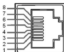
It provides two RS485 interfaces, loop out. Support for cascade connection and IMD remote control. The comparison of pins and Input connectors for RS485 is shown as in Table 4.2-1:
