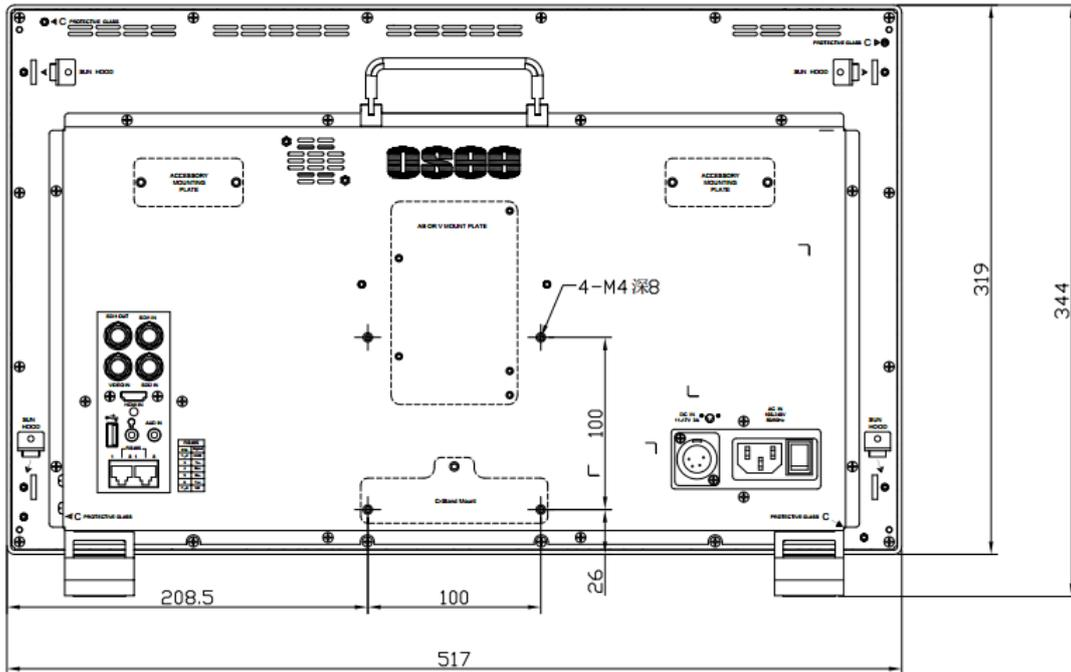
**Figure 6-2 Rear Panel(Unit: mm)**
