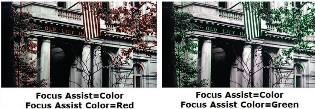
*Figure 5.1-21 Illustration for FOCUS ASSIST Function*
