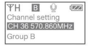
Use the + or - button to select the same channel as the receiver, and confirm it by short pressing the SET button.
