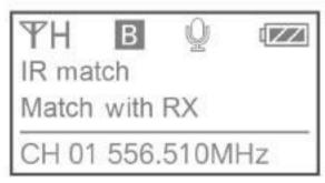
IR Match: Set to match with the receiver. The screen will display "Matching" when in process. After successful matching, it will read Match success. If failed to be matched within 20s, the screen displays "Match time out"
