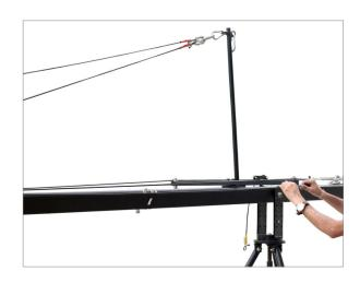
Now attach small 2 hooks at the back side of cable guide support rod .
