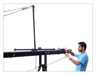
Align the cable to the cable guide from side and adjust the cable with help of wire tensioner. Same approach apply at other side of jib
