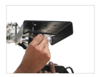
Mount your camera setup onto camera plate on Sr. pan tilt head with the screwed knob on the base.
