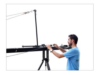
Now connect 9.7ft cable (cable code: blue) with the hook on section 3 of jib & attach it to the hook on section 6 (slot 2)of the jib
