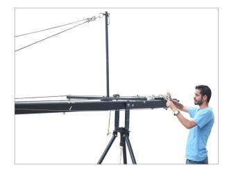
Align the cable to the cable guide from side and adjust the cable with help of wire tensioner. Same approach apply at other side of jib
