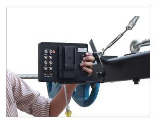
• Loosen the knob on joystick control in order to attach it to weight bar.
