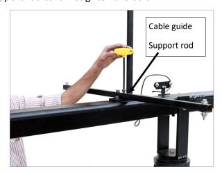
• Remove the threaded pin on head platform in order to install the Head Platform assembly (leveling arm up) to the end of the smallest section (front section) with the provided bolt, shaft collars, washers and nut.
