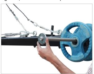
• Loosen the knob on rear section, remove closers from weight bar and insert it to slot on rear section.
