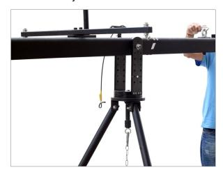
Attach 2 big hooks on both slots on cable guide. Then attach two extra hooks to big hook that is attached to front side and two hooks to hook that is attached to back side.
